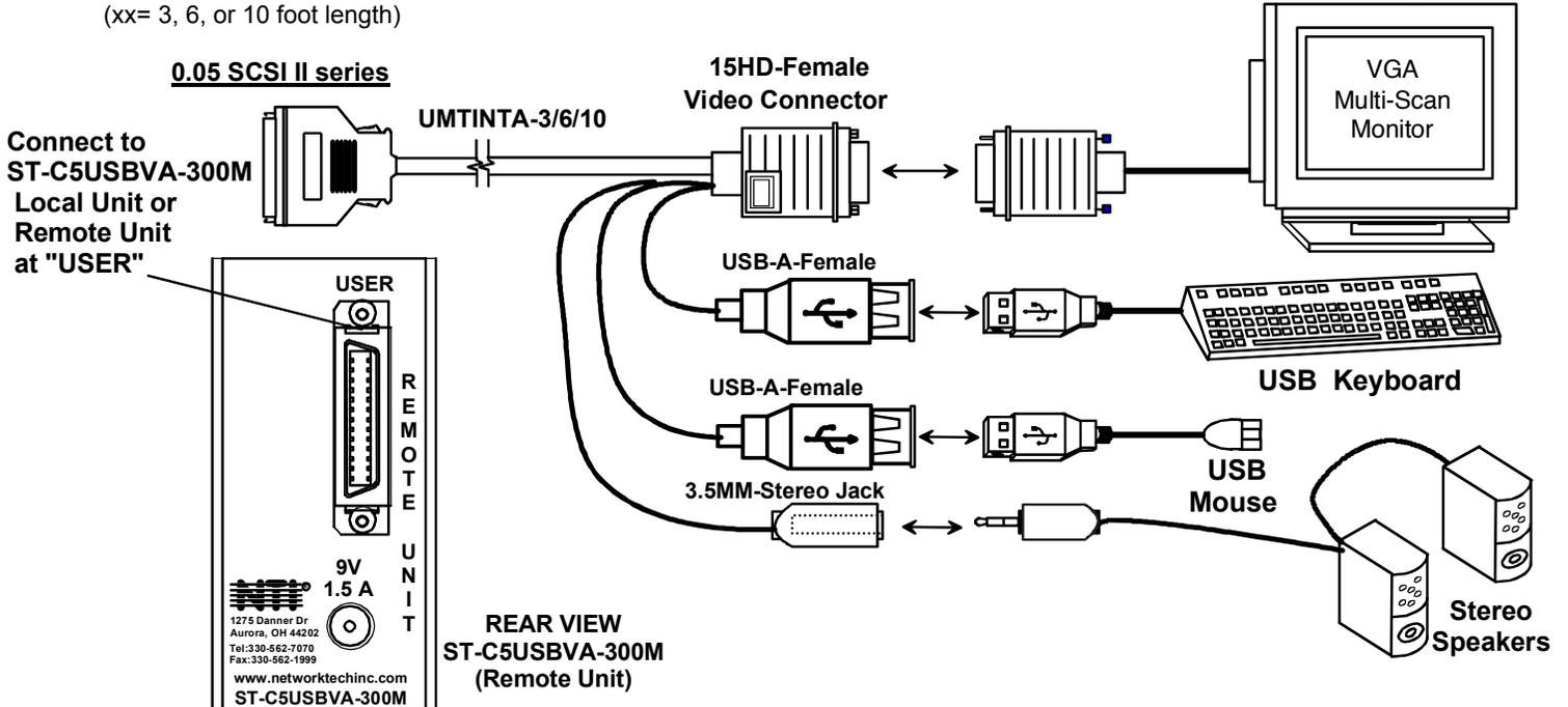
Figure 13- Connect cable between user and module
