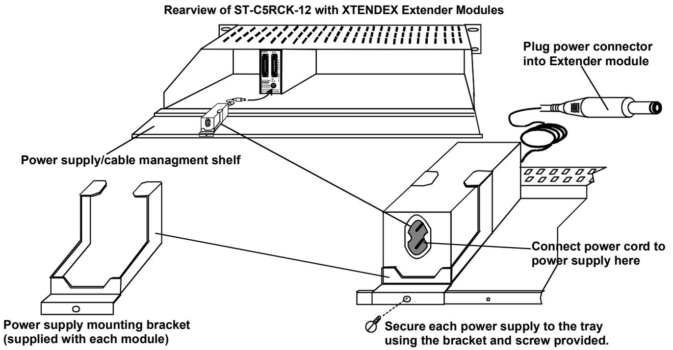
**Figure 11- Secure each power supply to the tray**
