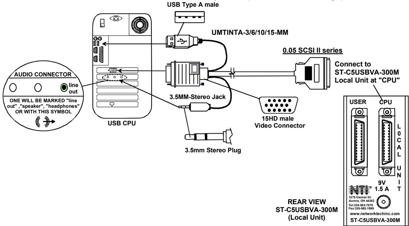
Figure 12- Connect cable between CPU and module
